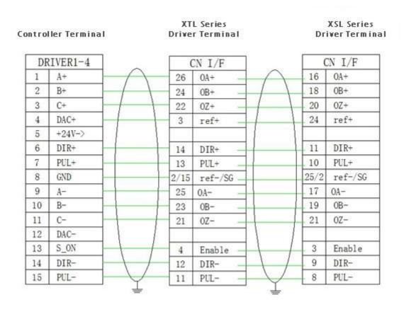
Please use shielded twisted pair cable It is recommended to use Misumi 8-core flexible cable Each core >= 0.3mm2, each core is composed of multiple copper wires 3367 3500
