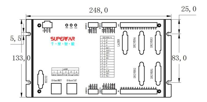
The QLC-420 control card is a high-end platform control card independently developed by Qianli Intelligent . It uses powerful CPU calculation and is mainly used in multi-axis motion platforms and laser processing applications.
